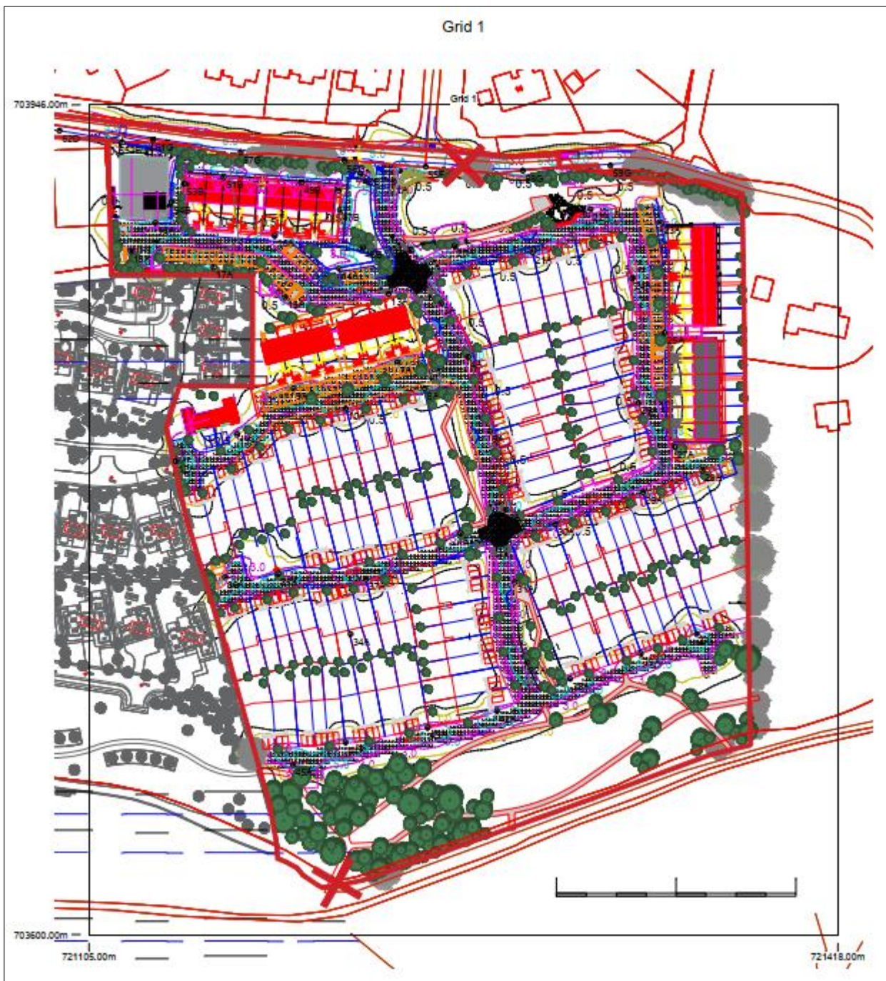
Figure 9d: Public Street Lighting layout (SES 15200 RevE.pdf - Source: Sabre Electrical Services Ltd., dated: 10/3/2021).
