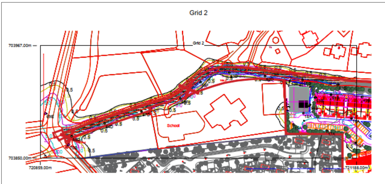
Figure 9e: Public Street Lighting layout along the Cookstown Public Road (SES 15200 RevE.pdf - Source: Sabre Electrical Services Ltd., dated: 10/3/2021).
